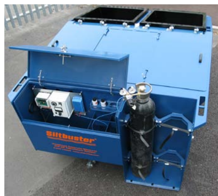
◀ The RCW unit accepts standard gas bottles
